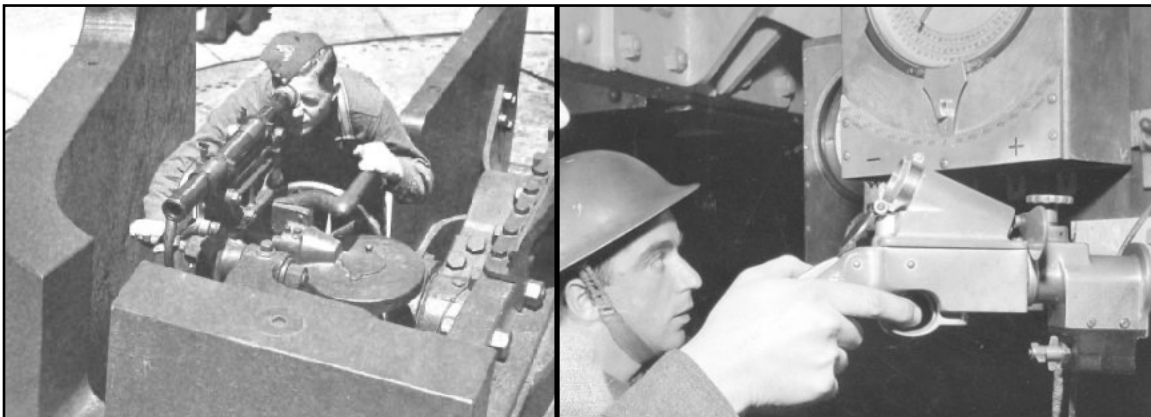
Left: the automatic sight fitted with a telescope. A cam attached to the sight bracket ensured the gun was at the correct elevation for the range when the telescope was laid on the waterline of the ship. Note the deep cut out in the forward shield for the sight. Right: The electric firing gear on a Mk 5 mounting. The bearing dial that was connected electrically to the battery plotting room can be seen in the upper right. LAC 399186 and 399242.
