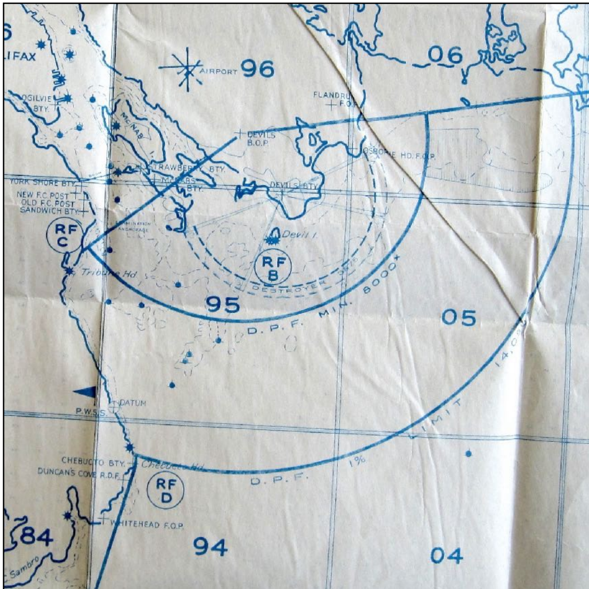
A diagram of the entrance to Halifax harbour with the arc of fire covered by Devils Battery. The outer arc is the limit of the depression position finder in order to obtain one percent accuracy in determining the range - about 14,000 yards (~12,800 m). Between them, Devils and Chebucto Batteries gave an effective cross fire at the entrance to the harbour. Fort Record Book.
